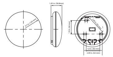
Fig. 1 - Wi-Fi Controller Dimensions
