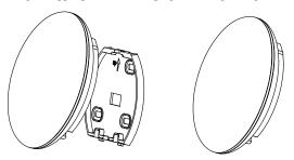
Fig. 11 — Reattaching the upper part of the Wi–Fi translator
