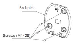
Fig. 7 — Mount the back plate to a wall
