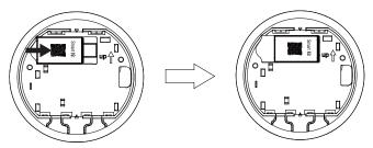
Fig. 6 - Insert Wi-Fi Dongle on USB Port
