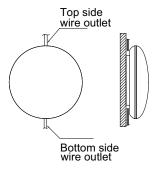
Fig. 8 — Exposed mounting
