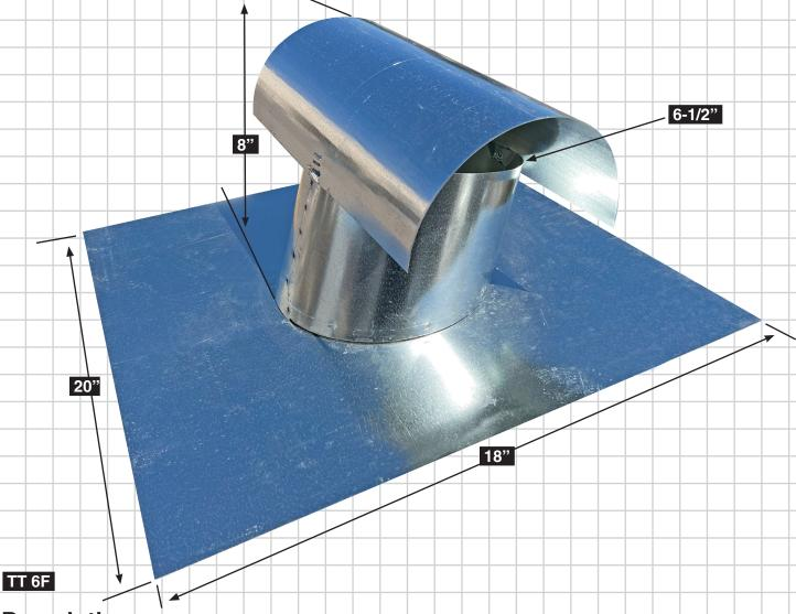
**Description:** 6 inch Roof Top vent. Fits 6 inch OD single wall duct pipes. All galvanized steel cone and top with a die formed galvanized steel base. Base has a 1/2" internal lip to prevent leakage. Internal wire screen version prevents rodents and bugs.
