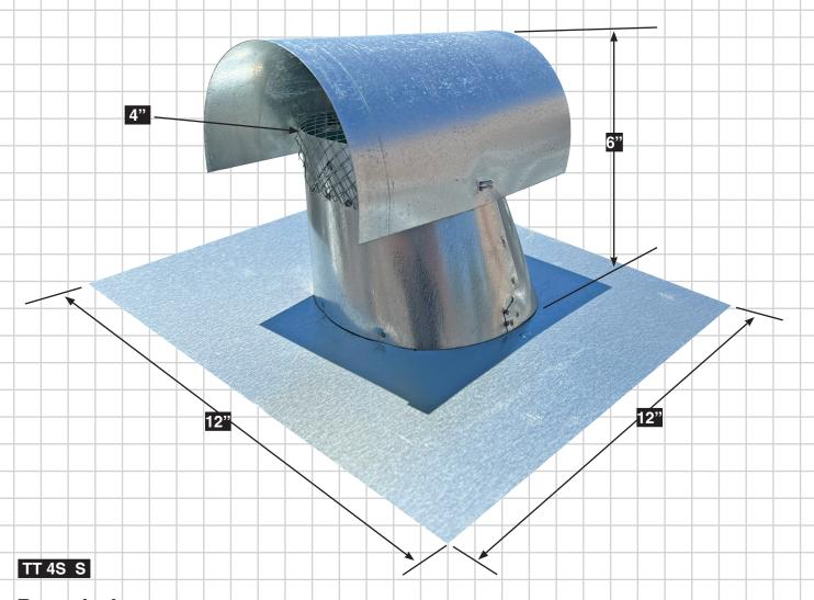
**Description:** 4 inch Roof Top vent. Fits 4 inch OD single wall duct pipes. All galvanized steel cone and top with a die formed galvanized steel base. Base has a 1/2" internal lip to prevent leakage. Internal wire screen version prevents rodents and bugs.
