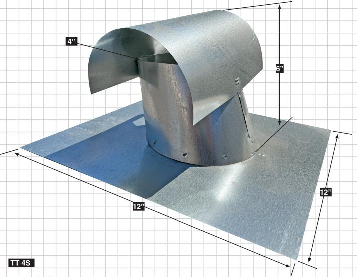
**Description:** 4 inch Roof Top vent. Fits 4 inch OD single wall duct pipes. All galvanized steel cone and top with a die formed galvanized steel base. Base has a 1/2" internal lip to prevent leakage. Internal wire screen version prevents rodents and bugs.
