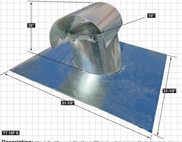
**Description:** 10 inch Roof Top vent. Fits 10 inch OD single wall duct pipes. All galvanized steel cone and top with a die formed galvanized steel base. Base has a 1/2" internal lip to prevent leakage. Internal wire screen version prevents rodents and bugs.
