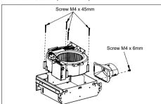
Using wire nuts (not provided) connect house wires to fan wires as shown in "CONNECT WIRING" diagram A. Insert housing into ceiling or wall opening and secure housing by using tapping screws (ø 4x25 mm).
