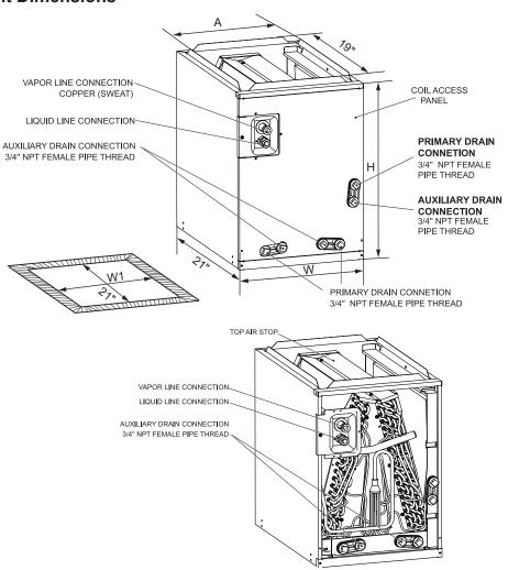
Fig.2-1 CASED DIMENSIONS AND COMPONENT LOCATION
