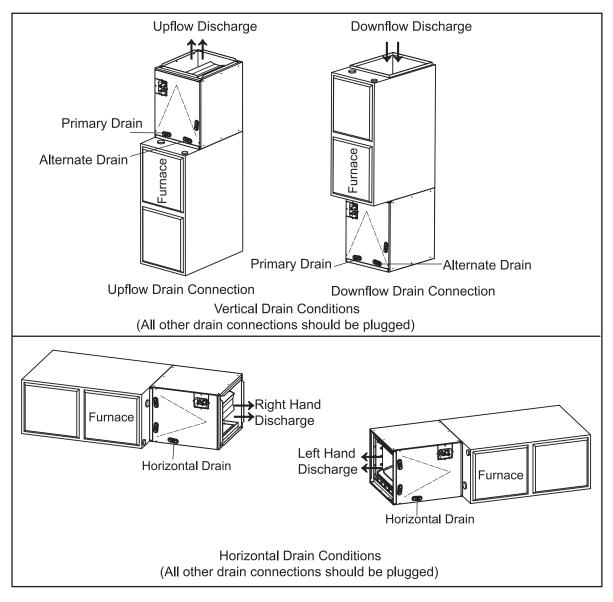
Fig. 3-1 INSTALLATION OF CASED COIL
