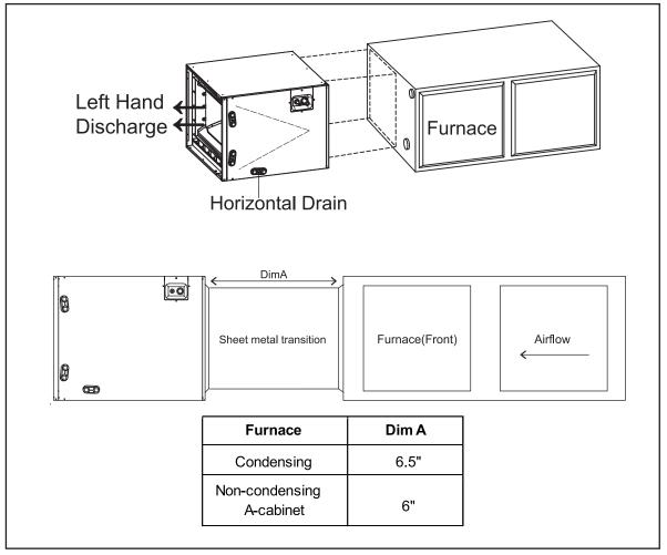
Fig. 3-2 Transition for horizontal left orientation
