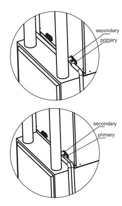
Fig. 4-2 DRAIN PIPE ROUTING
