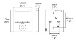
Fig. 1 — Wired Remote Controller Dimensions
