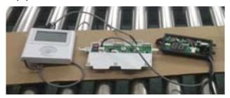
Fig. 16 - Wired Controller, Adapter Board, and Display Board
