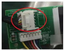
Fig. 18 - CN101 Connection to the Adapter Board
