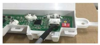
Fig. 23 - Adaptor Board to Display Board Connection
