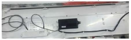
Fig. 26 - Front Panel with New Display Board and Adapter Board
