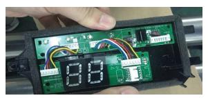
Fig. 21 - Display Board Installed on the Display Board Holder
