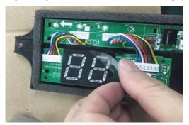
Fig. 22 - Display Board Screen Cover
