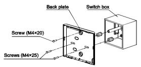
Fig. 6 — Flush Mounting
