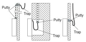
Fig. 11 - Seal the wires
