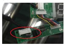
Fig. 17 - CN201 Connection to the Main Control Board
