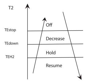
**Fig. 19 – Evaporator Coil Temperature Protection** NOTE:
