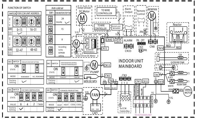
Fig. 6 – Wiring Diagram Sizes 9K–24K
