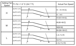
Fig. 16 - Indoor Fan Running Rules
