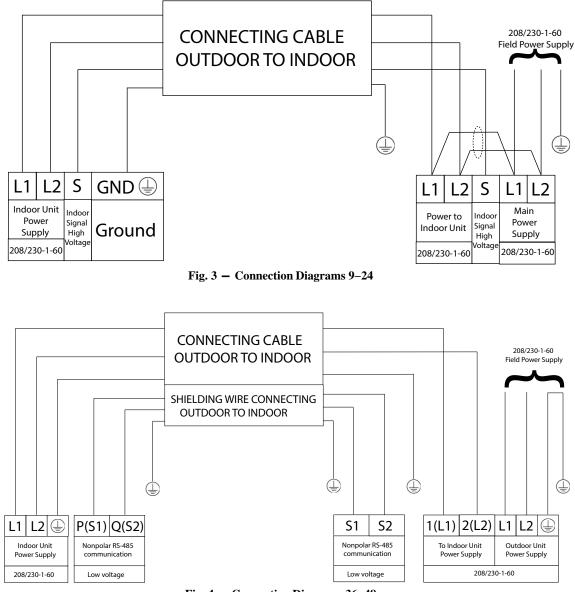
Fig. 4 - Connection Diagrams 36–48
