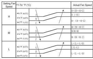
Fig. 14 - Indoor Fan Running Rules
