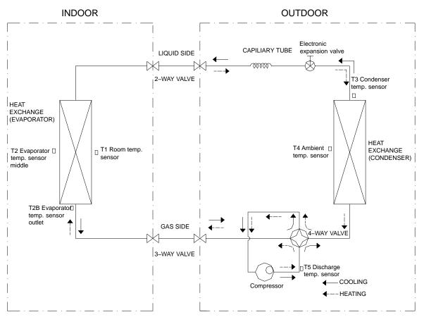
Fig. 8 - Refrigerant Cycle Diagram
