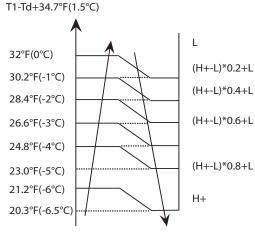
Fig. 17 – Auto Fan Action in HEATING Mode
