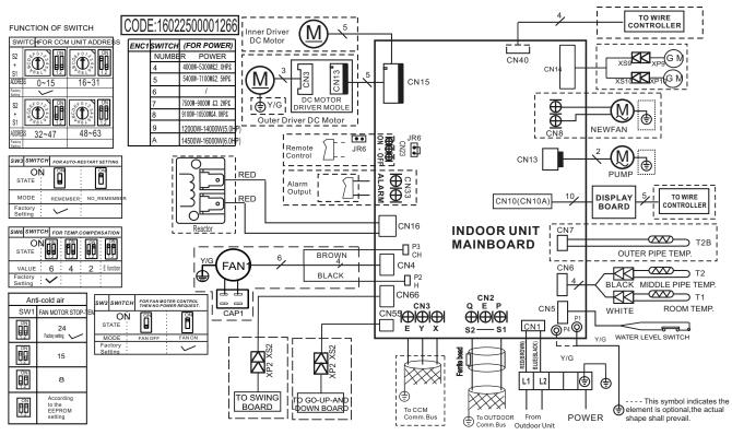
Fig. 7 - Wiring Diagram (Size 36K-48K)
