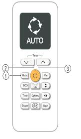
AUTO Operation SETTING TEMPERATURE The operating temperature range for units is 62°F - 86°F (17°C - 30°C). You can increase or decrease the set temperature in 1°F increments. In AUTO mode, the unit will automatically select the COOL, FAN, HEAT or DRY mode based on the set temperature. 1. Press the MODE button to select the AUTO mode. 2. Set your desired temperature using the TEMP V or 2 TEMP / button. 3. Press the ON/OFF button to start the unit.
