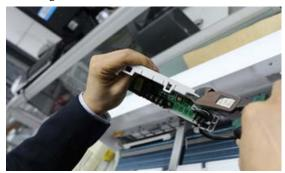
Fig. 28 - Cut a hole on the multi-function board
