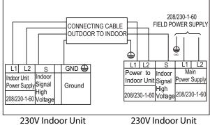
Fig. 17 — Connection Diagrams
