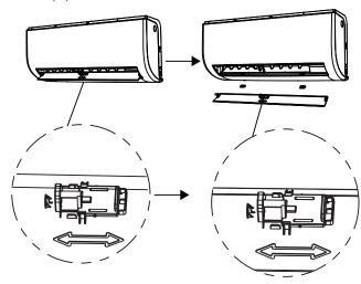
Fig. 13 — Disassemble the Louver
