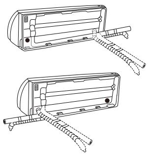
Fig. 11 - Piping Angle
