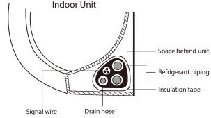
Fig. 19 - Bundle drain hose, refrigerant pipes, and signal cable
