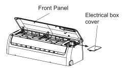
Fig. 11 - Terminal Block Location
