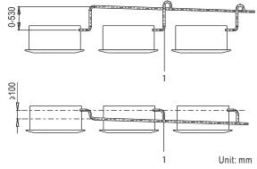
1 T-joint converging drain pipes
