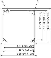
Fig. 4 - Drilling Holes
