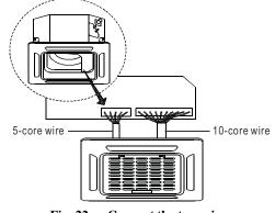
Fig. 22 – Connect the two wires
