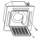
Fig. 24 - Fasten the Control Box Lid
