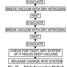
Fig. 32 - Triple Evacuation Method
