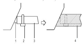
Fig. 12 - Push the Drain Hose
