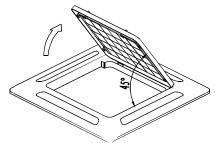
Fig. 18 - Open Intake Grille
