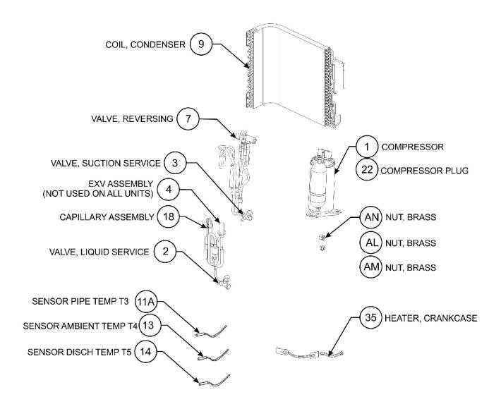
Note: This illustration is for reference only. Your unit may differ in appearance or may not include all components shown. COIL, PIPING & COMPRESSOR PARTS
