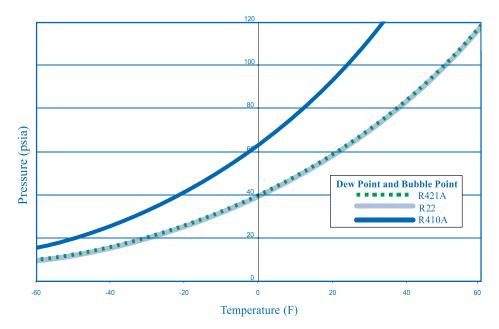
**R421A** is a HFC blend replacement with zero ODP and is compatible with both synthetic and mineral oils.
