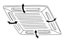
There will be water condensing on the louvers if setting the louvers down when cooling. (Cassette type only)
