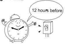
To protect the compressor, please turn on the power switch 12 hours before starting the unit. •
