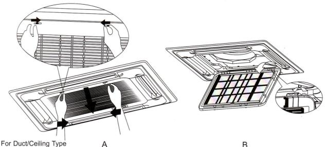
Push the grill switches to the arrow directions, then open the air-in grill downwards. T
