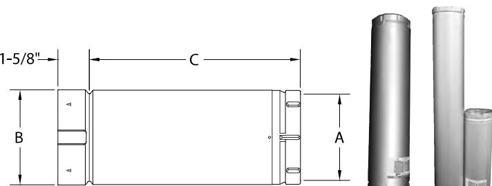
**NOTE:** Dimension C is installed length. Nominal length is 60".
