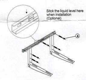
PS: Please check and make sure connecting screws should be tightened on the bracket after finished installation
