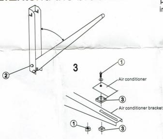
4. Fix bracket to the wall using the holes provided in the bracket to complete installation.
